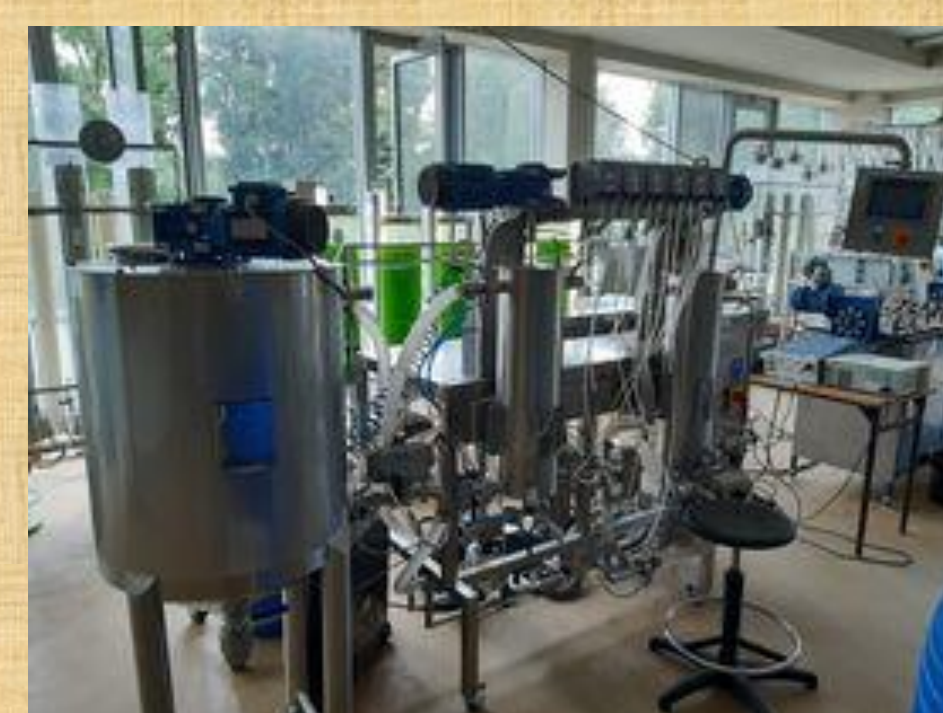
Figure. 1 The laboratory installation for drainage treatment operating based on biomass attached to the filling (biofilm)
